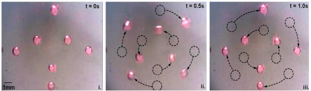
Figure 6: Parallel movement of droplets. 7 droplets undergo simultaneous movement.4 outer droplets moves clockwise in a circular manner, whilst 3 inner droplets move anti-clockwise in a circular manner (50 Vppk, 10 kHz).
