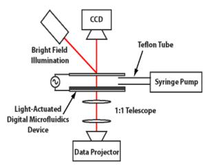
Figure 2: Experimental setup. A standard data projector (spatial light modulator) is focused onto the light-actuated digital microfluidics substrate with a 1:1 telescope. Bright-field illumination and a CCD camera allow for droplet visualization.
