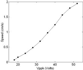
Figure 3: Maximum droplet speed versus voltage for a 200 nL droplet at 10 kHz frequency.
